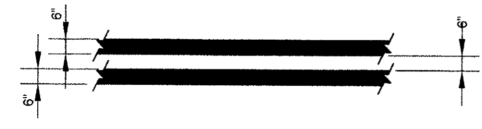
FULL YELLOW BARRIER LINE (FYBL) (YELLOW) N.T.S.
