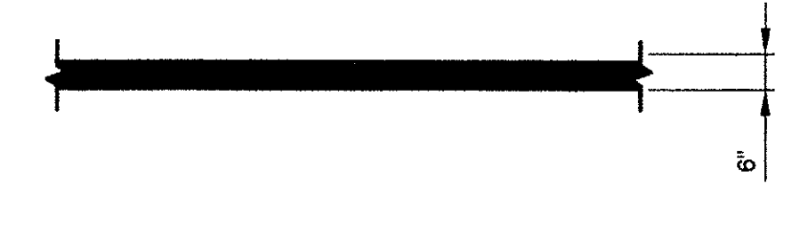
SOLID PARKING STALL LINE (SWPSSL OR SBPSSL) (WHITE OR BLUE) N.T.S.
